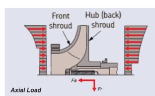
The axial hydraulic pressures acting on a single stage centrifugal pump are illustrated in the figure. The axial load is equal to the sum of the forces.
