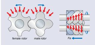
The gas pressure is low at the suction side and higher at the discharge side. The gas pressure along the length of rotor produces radial forces and axial forces from the pressure acting on the projected areas. The net axial force always towards to the suction side.
